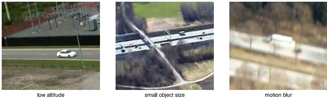
Fig. 6.1: Examples images taken from aerial platforms. Images can be recorded from low (left) or high (center) altitudes resulting in different viewing angles and object sizes. Viewing objects from far distances and fast camera motion may produce artifacts such as motion blur in the images (right).
