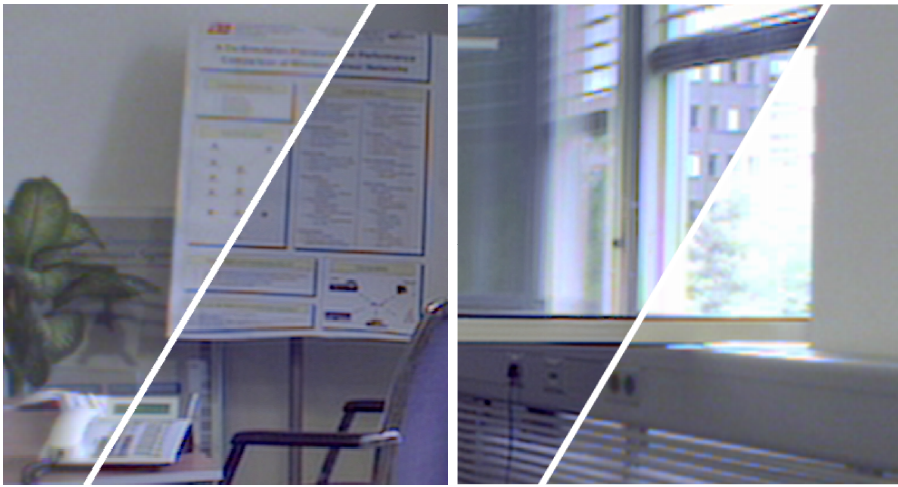
Fig. 4.13: Zoomed views: Comparison of low-resolution image captured with auto exposure setting (bicubic interpolated: left part of left image and right part of right image) and proposed enhancement.
