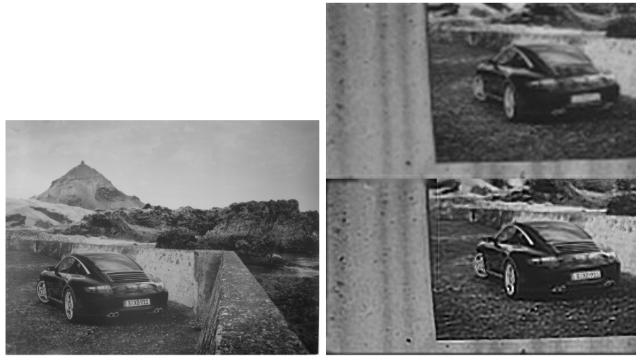
Fig. 3.15: Left: high-resolution still image, Right-Top: bicubic interpolated low-resolution video frame, Right-Bottom: MAP superresolution with Huber-prior and high-resolution prior.
