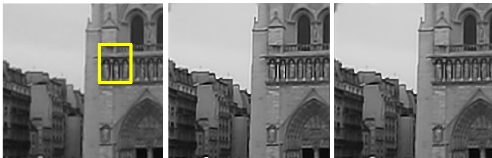
Fig. 3.9: Left: Bicubic interpolation of low-resolution input, Middle: MAP superresolution using Huber-prior, Right: MAP superresolution with Huber-prior and high-resolution prior.
