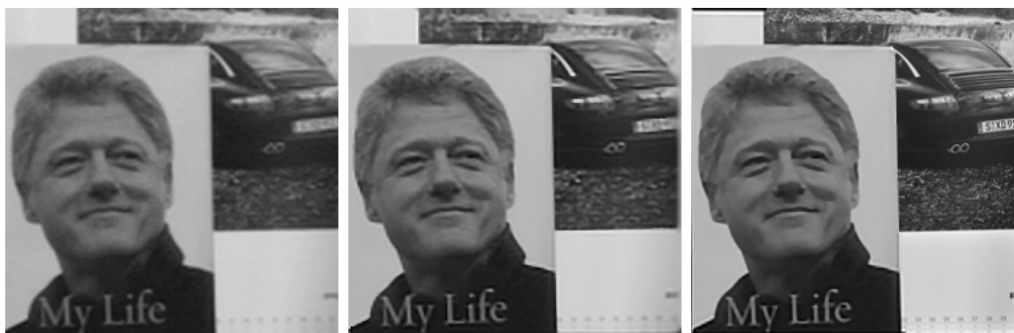
Fig. 3.13: Left: Bicubic interpolation of low-resolution input, Middle: MAP superresolution using Huber-prior, Right: MAP superresolution with Huber-prior and high-resolution prior.
