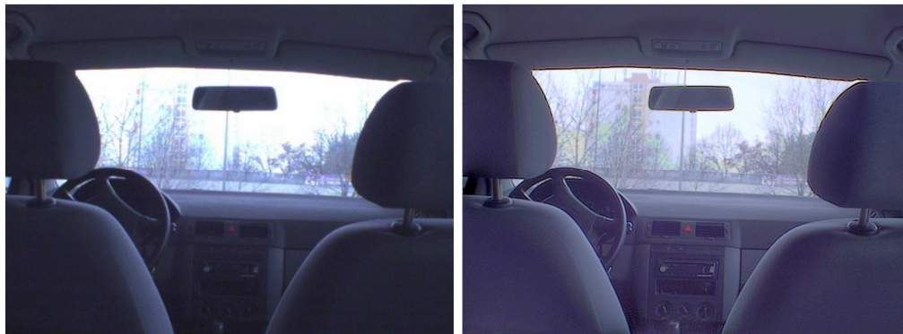
Fig. A.13: Comparison of low-resolution image captured with auto exposure setting (bicubic interpolated, left) and proposed enhancement (right).
