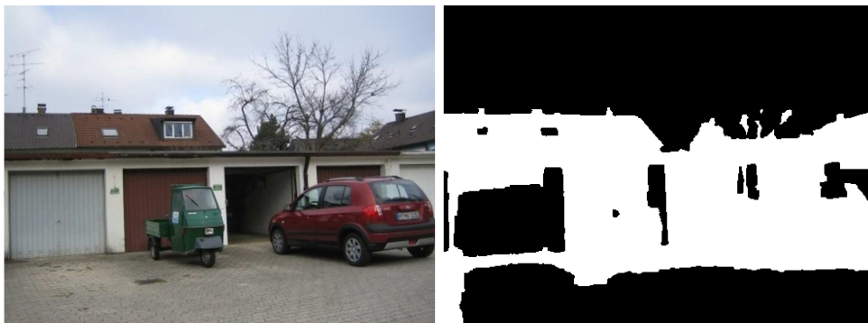
Fig. 4.5: Example mask (right) corresponding to input (left) and results shown in Fig. 4.15: in black areas pixels are transferred from the image with short exposure time and in white areas the image with long exposure time is used instead.
