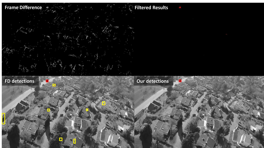
Fig. 6.10: Binary maps and detections of sequence 5 for frame-differencing approach (left) and our approach (right).
