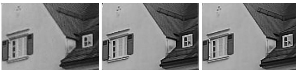
Fig. 3.14: Left: Bicubic interpolation of low-resolution input, Middle: MAP superresolution using Huber-prior, Right: MAP superresolution with Huber-prior and high-resolution prior.
