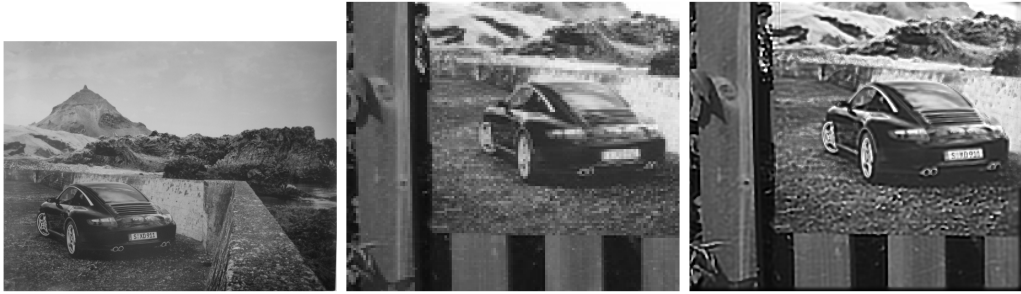
Fig. 3.11: Left: high-resolution still image, Middle: low-resolution video frame, Right: MAP superresolution with Huber-prior and high-resolution prior.
