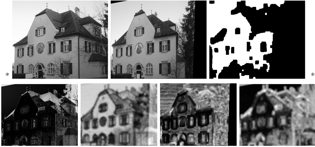
Fig. 3.6: Top: Aligned sample input images (Left: first video frame, Right: still image). Bottom: different dissimilarity images between inputs (Left-Right: SSD, MI, NCC, HOG).
